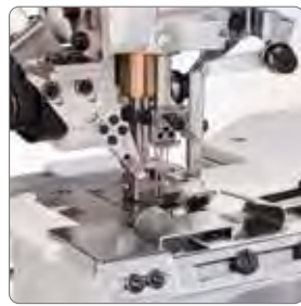
CHP (CRL 163) 氣動式下擺車縫 Pneumatic Hemming
